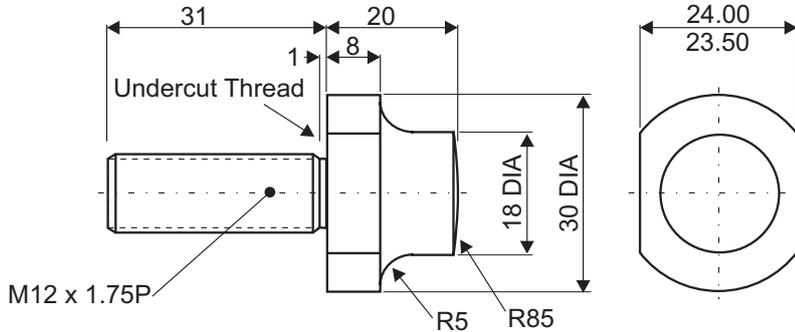
**GKLB-12S Load Button with M12 Thread**
