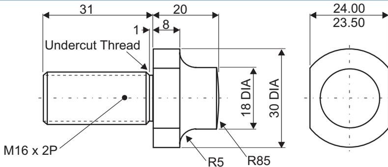
**GKLB-16S Load Button with M16 Thread**
